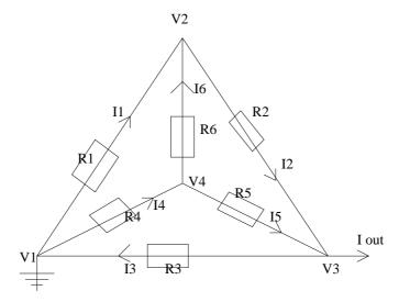
Write down in matrix form the voltage drops as a function of voltages, the currents as a function of voltage drops, and the conservation of currents. Lastly write down system of equations from which the voltages can be determined.
